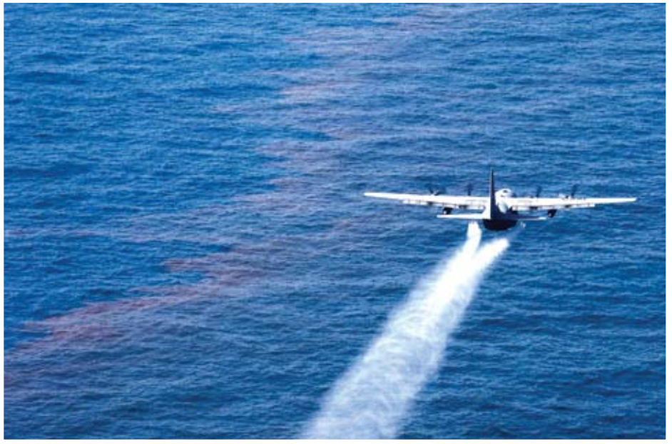
A C-130 Hercules from the Air Force Reserve Command's 910 th Airlift Wing drops an oil-dispersing chemical into the Gulf of Mexico as part of the Deepwater Horizon Response effort. (Source: US Air Force via Wikipedia.)
